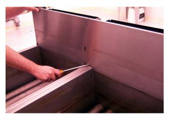
Removing flue cap.
